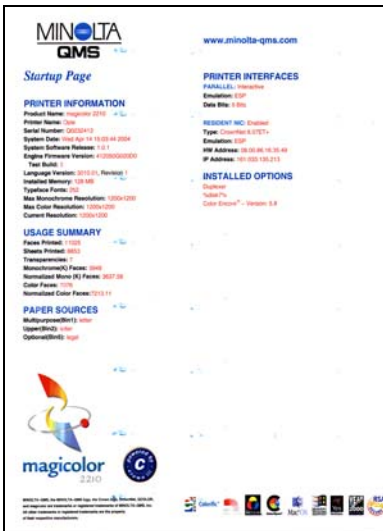
Note the line of defects that repeat down this magicolor 2210 startup page. This is caused by damage to the developing roller in the non-genuine KONICA MINOLTA cyan toner cartridge.
