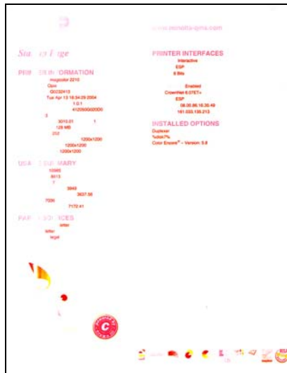
The developing rollers in these non-genuine KONICA MINOLTA cyan and black toner cartridges locked up, causing only yellow and magenta to be printed on this magicolor 2210 startup page.
